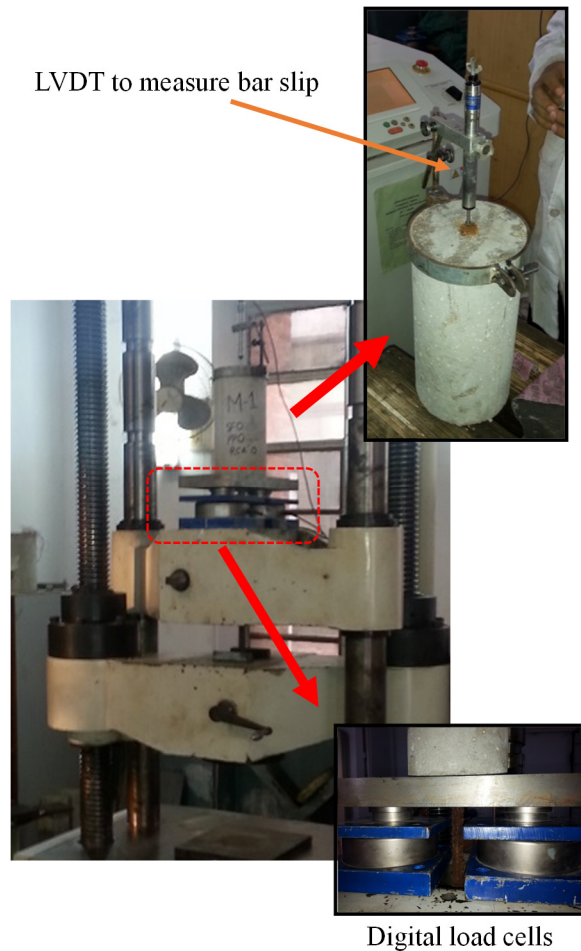
Fig. 8: Testing Arrangement for Pull-Out Test
